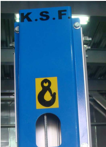
cable under steel crank-case and crane lifting point for safe transportation
